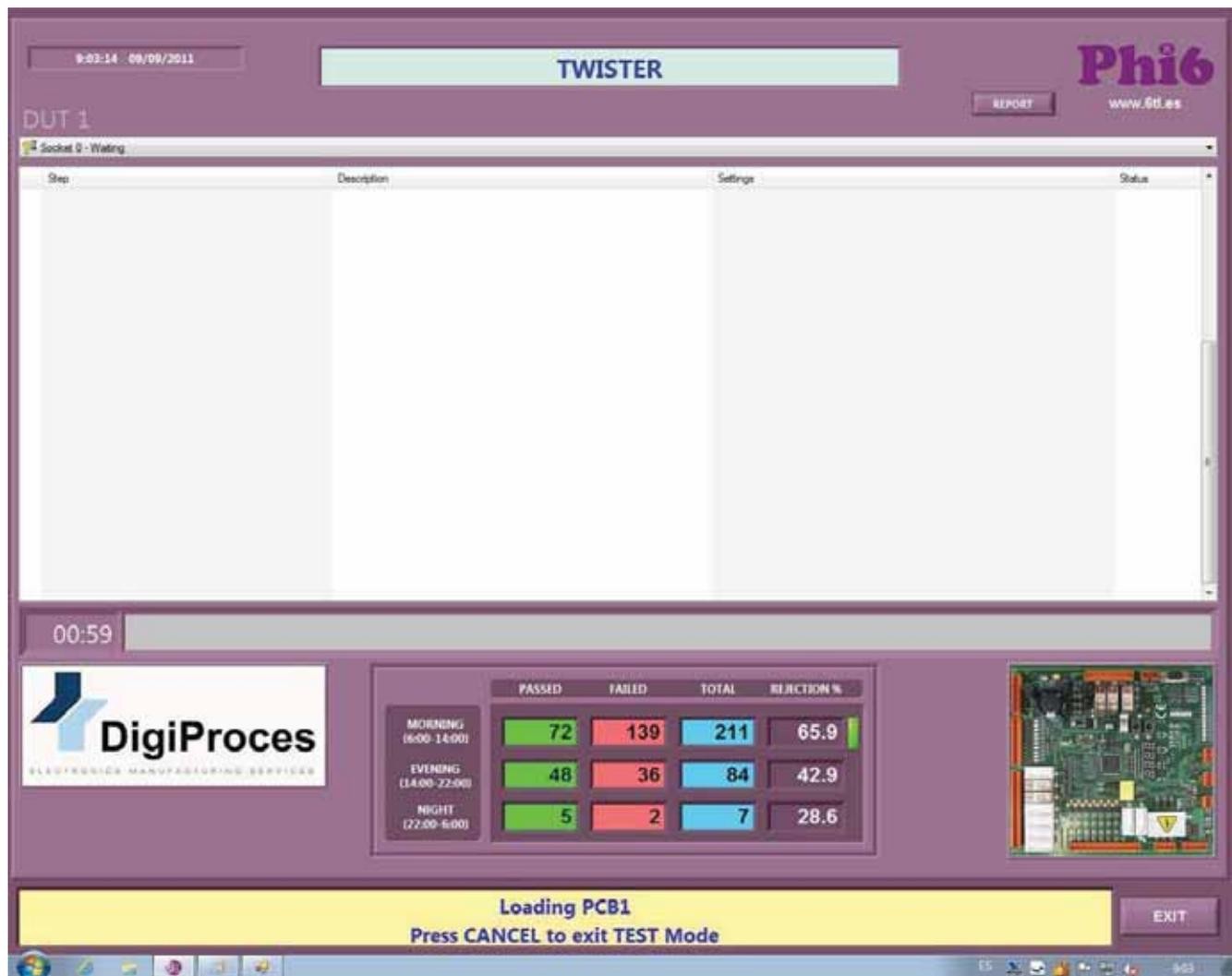
The sequence execution is displayed as well as metrics of passed, failed and total devices been tested.
