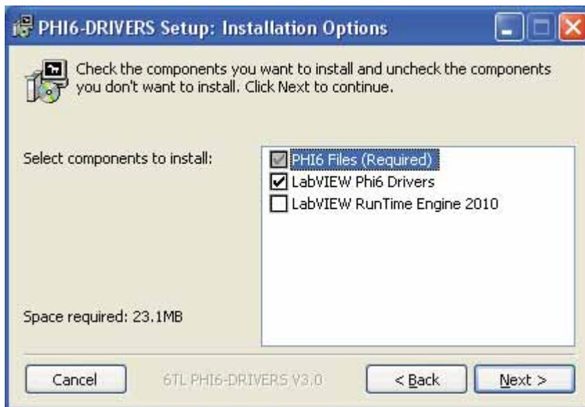
1. *PHI6 Files*: installs the Phi6 Explorer (always required).
