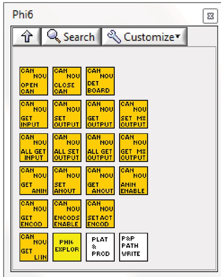
4. **Open Phi6:** Opens CAN communication to the YAV boards. Needed at the beginning of an application before any YAV operation is executed (See Phi6 Template).
